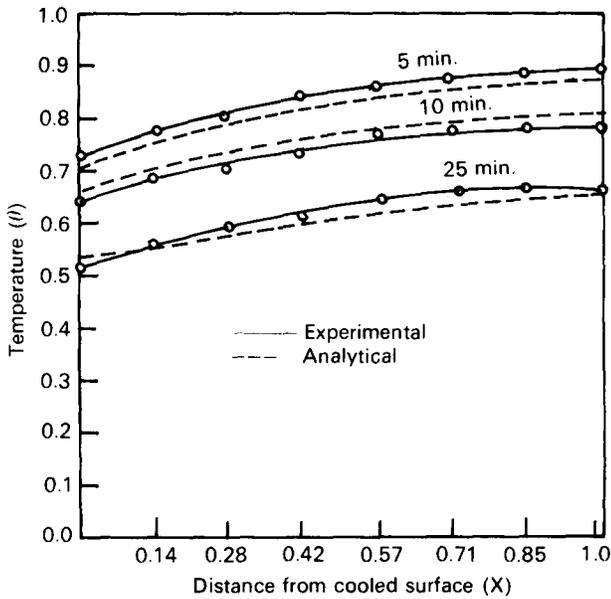
Figure 2 Temperature profiles for solidification of 50-50 tin-lead alloy
